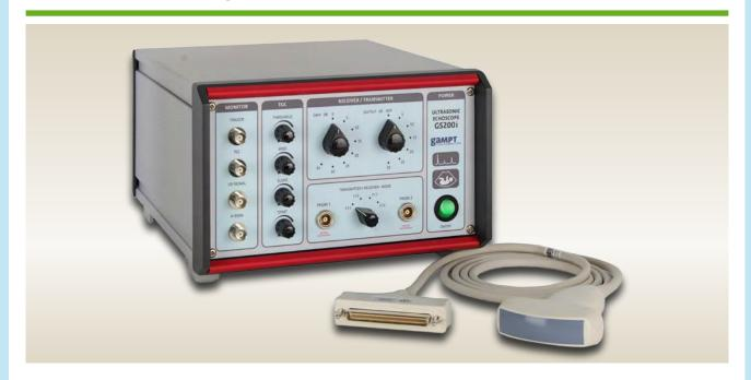
The GS200i is a high-resolution ultrasonic measurement system based on the GS200 (order no. 10400). With this device ultrasonic measurements can be made with the single-element transducers (order no. 10151-10154) and ultrasonic images can be produced using the B-mode and M-mode methods with an ultrasonic array transducer.
