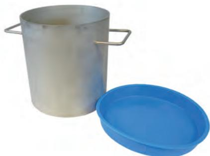
**10.0031 NF EN 480-4 - XP P18-468****CYLINDRE POUR LA MESURE DU RESSUAGE DU BÉTON**
